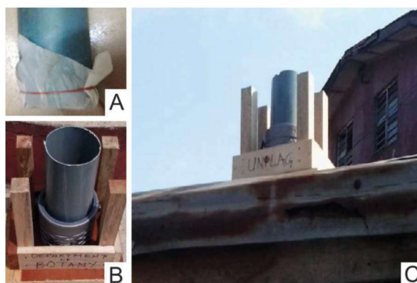
Modified Gbenga-2 aerosampler. A. Sampler cylinder with 5 µm sieve. B. Sampler setup complete in UniLag. C. Mounted sampler on 2 m high shop in Ebute-Metta.
