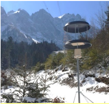
The gravimetric pollen trap located near Eibsee Alm (1016 m a.s.l.).
